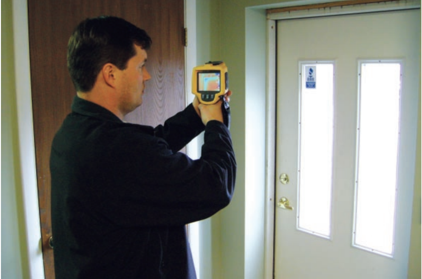
True Energy Solutions in Rochester, New York checks for drafts with an infrared camera as part of a free energy audit it provides to qualifying households. The company is reimbursed with funds from polluter-purchased emissions credits through the Regional Greenhouse Gas Initiative.
